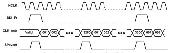
Figure 3–2. Source Packet Transmit Event Timing
