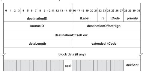
Figure 3-34. Block-Receive Format for Control FIFO
