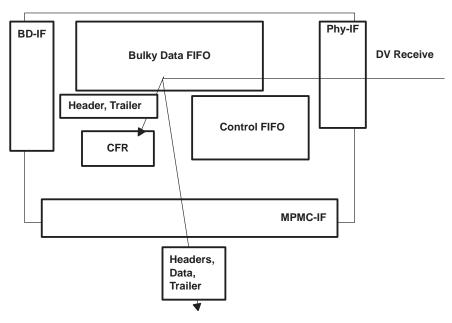
Figure 3-22. Header, Data, and Trailer Received at MP/MC
