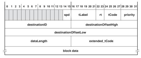
Figure 3-31. Block-Transmit Format
