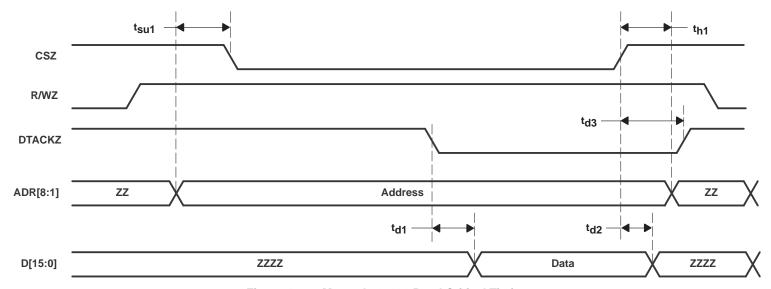
Figure 4–28. Motorola 68000 Read Critical Timing
