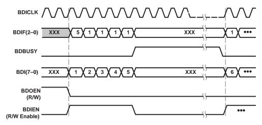
Figure 4–13. Functional Timing for Write Operations in Bidirectional Mode
