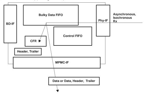
Figure 3-20. Receive Asynchronous/Isochronous Data to Microprocessor Interface
