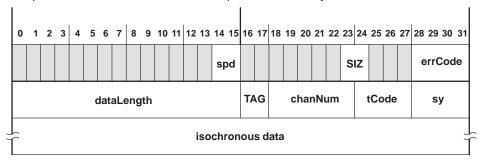
Figure 3-37. Isochronous-Receive Format for Bulky Data FIFO
