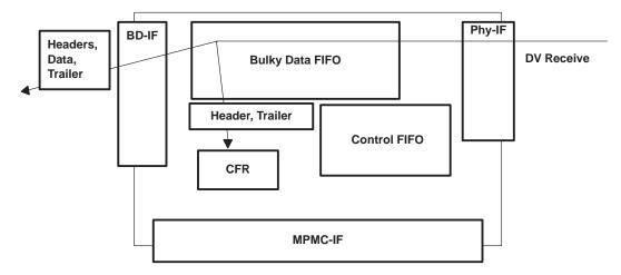
Figure 3-21. Header, Data, and Trailer Received at BDIF
