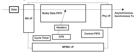
Figure 3–10. Transmit Asynchronous/Isochronous Data from BATX by the Bulky Data Interface with Auto-Packetization
