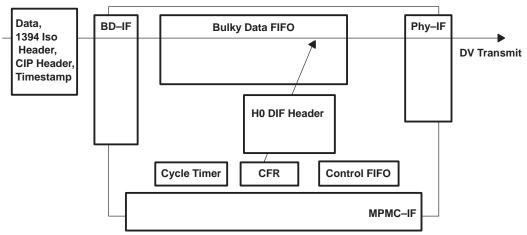
Figure 3-16. Data 1394 Isochronous and CIP Headers
