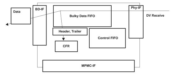
Figure 3-23. Header, Trailer Stripped, Data only sent to BDIF
