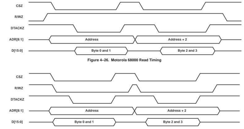
Figure 4–27. Motorola 68000 Write Timing
