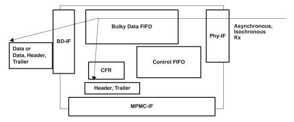
Figure 3-19. Receive Asynchronous/Isochronous Data to Bulky Data Interface
