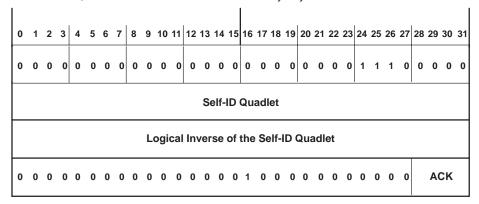
Figure 3-41. Receive Self-ID Format for Broadcast Write Receive FIFO
