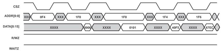
Figure 4-24. TMS320AV7100 ARM Blind Access Mode Read Timing
