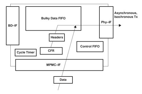
Figure 3–11. Transmit Asynchronous/Isochronous Data from BATX by the MP/MC Interface with Auto-Packetization
