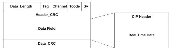
Length field is either 488 bytes (DV-Source Packet) or 8 bytes (empty packet).
