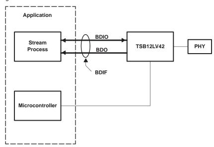
Since the BDIF has two ports data can be full duplex. One port is bidirectional and the other is output only. Each port has its own independent clock, control signals, and modes of operation. The ports can operate in asynchronous clock domains.
