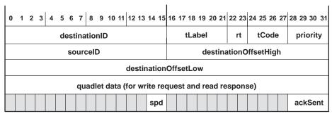
Figure 3-32. Quadlet-Receive Format for Control FIFO
