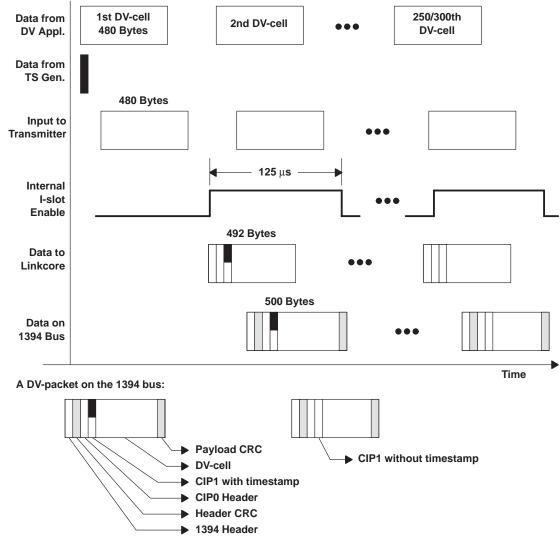
Figure 3-3. DV Packet on 1394 Bus
