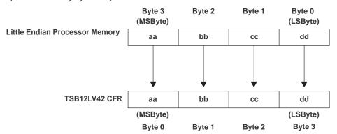
Figure 4-36. Little Endian Data Invariant System Design Illustration Chart
