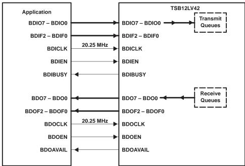
Figure 4–3. Bulky Data Interface Mode A Typical Application
