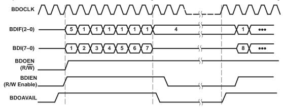
Figure 4-15. Functional Timing for Read Operations in Bidirectional Mode
