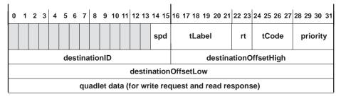
Figure 3-30. Quadlet-Transmit Format
