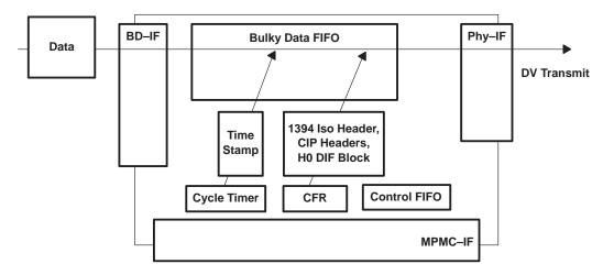
Figure 3-14. Data from Bulky Data Interface, Headers/Timestamp/H0 Automatically Inserted
