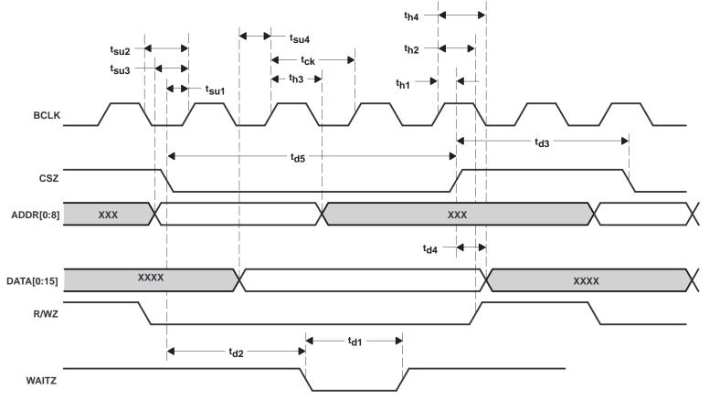
Figure 4–21. TMS320AV7100 ARM Read/Write Critial Timing
