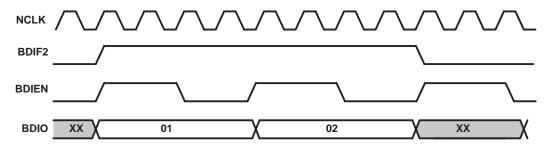
Figure 4-9. Functional Timing for Write Operations in the Asynchronous Mode
