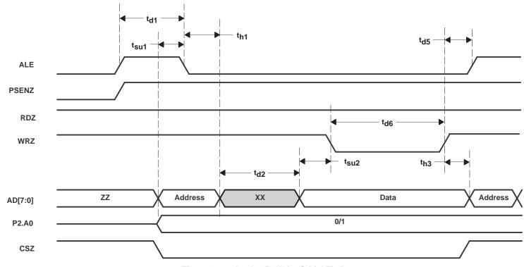
Figure 4–33. Intel 8051 Write Critial Timing
