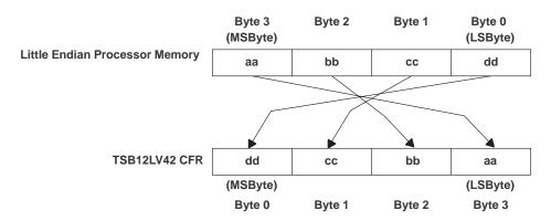
Figure 4-37. Little Endian Address Invariant System Design Illustration Chart
