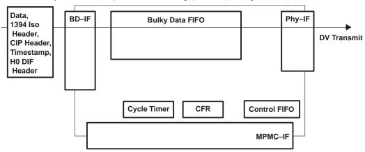
Figure 3-17. All Data from BDIF, including 1394 Isochronous Header
