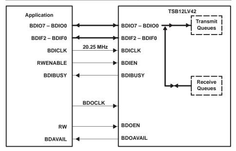
Figure 4-6. Bulky Data Interface Mode D Typical Application
