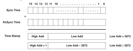
Figure 3-29. Time Stamp Determination on Receive
