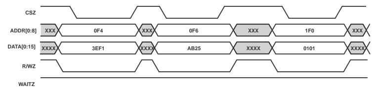
Figure 4-25. TMS320AV7100 ARM Blind Access Mode Write Timing
