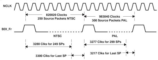
Figure 3-1. Example of a Source Packet Transmit Event
