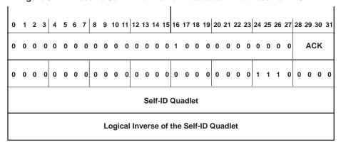
Figure 3-42. Receive Self-ID Format for Bulky Asynchronous Receive FIFO
