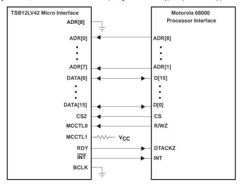
Figure 4–17. DVLynx Connections for 68000 Microcontroller
