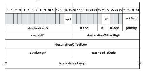
Figure 3-35. Block-Receive Format for Bulky Data FIFO
