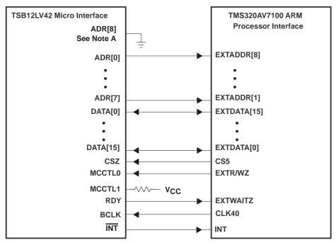
NOTE A: Connect as shown for 16-bit data. If 8-bit data bus is being used then connect ADR[8] on the TSB12LV42 to EXTADDR[0] on the TMS320AV7100.
