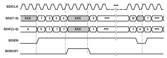
Figure 4-7. Functional Timing for Write Operations in the Unidirectional Modes
