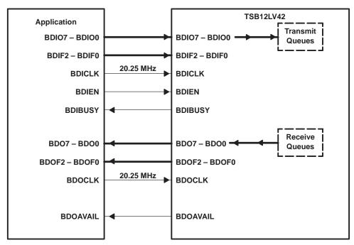
Figure 4-4. Bulky Data Interface Mode B Typical Application
