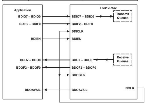
Figure 4-5. Bulky Data Interface Mode C Typical Application
