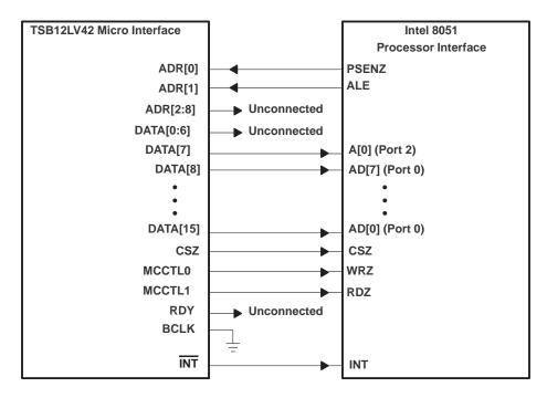
Figure 4-18. DVLynx Connections for 8051 Microcontroller
