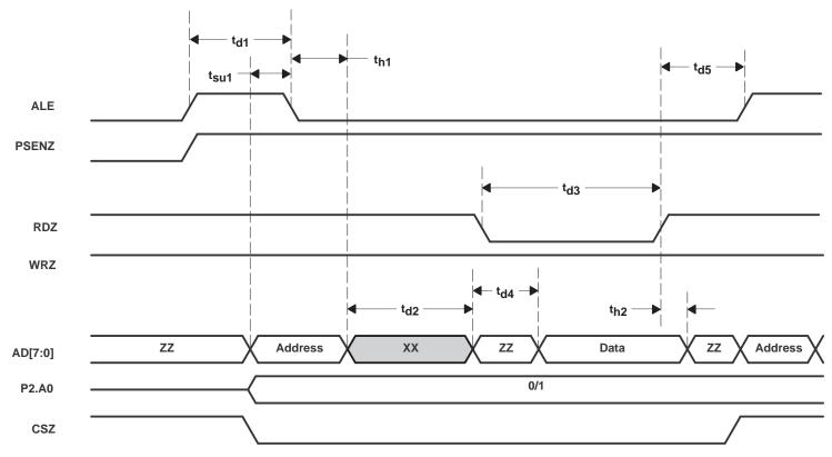
Figure 4–32. Intel 8051 Read Critial Timing
