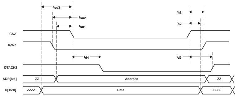
Figure 4–29. Motorola 68000 Write Critical Timing
