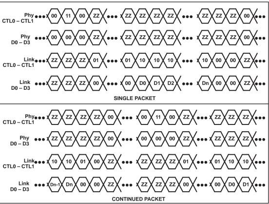
NOTE A: ZZ = high-impedance state, D0 - Dn = packet data
