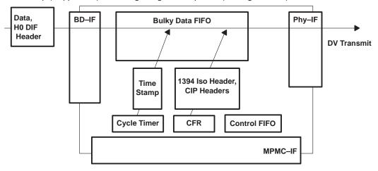
Figure 3–15. Data and H0 Header from Bulky Data Interface, Headers/Timestamp Automatically Inserted
