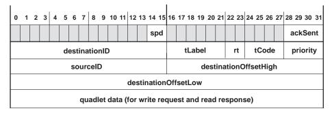
Figure 3-33. Quadlet-Receive Format for Bulky Data FIFO
