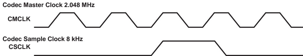
Figure 4–5. Codec Master and Sample Clock Timing
