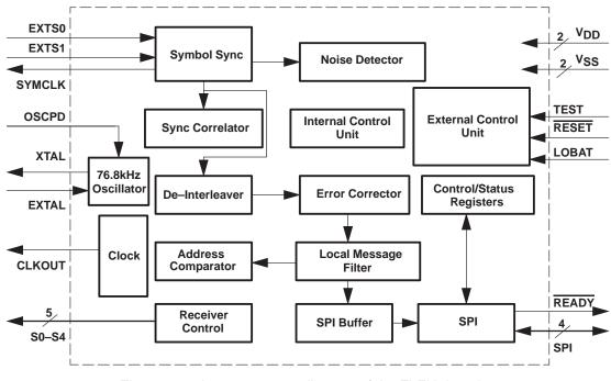
Figure 3–2 shows a system diagram of the FLEX decoder.
