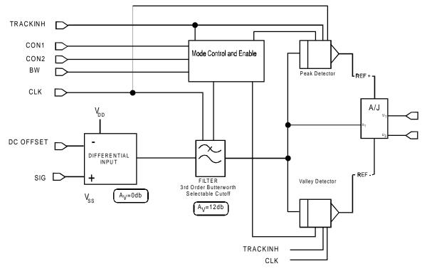
The analog inputs to the TLV5590 are DC offset voltage and the baseband audio signal. Both of these analog inputs <u>may</u> be received from the IF IC. The DC offset voltage is used to set the midpoint of the dynamic range for the TLV5590 to ensure that no signal clipping will occur. The DC voltage applied to OFFSET is subtracted from the SIG pin to minimize the receiver offsets.
