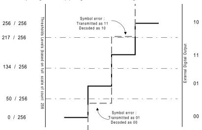
Figure 7. Bit Errors Caused by Signal Clipping of FILOUT Signal
