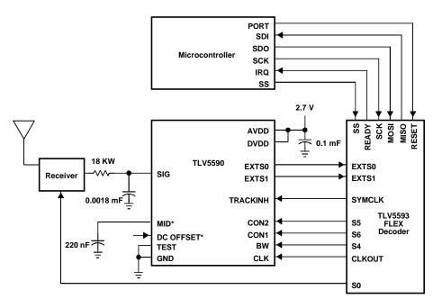
The voltage on the MID terminal is nominally AVDD/2. The voltage applied to the DC OFFSET terminal is set to the dc offset voltage of the input signal applied to the SIG ter
