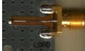
Figure 2. Placement of the Resistor at the end of the Transmission Line
