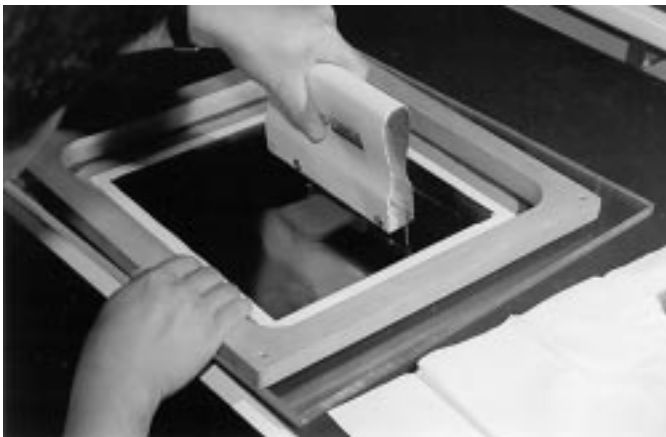
Figure 2. Solder Is Screened Onto the Ceramic Substrate
