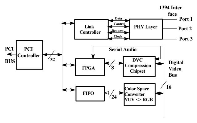
Fig4: 1394/DV adapter-codec block diagram
