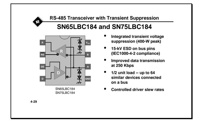
The SN65/75LBC184 is the industry's first '176 standard footprint 485 differential transceiver to offer integrated transient voltage protection up to 400-W peak. The SN65/75LBC184 provides significant protection from large over-voltage transients on the bus pins, which can be caused by secondary effects of a lightning strike or power system switching disturbances.
