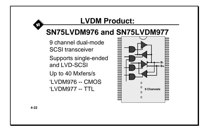
TI's LVDM products are the ultimate solution to multiplex and half-duplex interconnections. These products enable bi-directional connections while still enjoying all the LVDS benefits. Their application usually includes any type of multipoint differential bus including proprietary buses, backplane systems and direct board-to-board connections.
