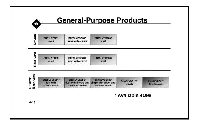
The above devices all fall under the category of general -purpose LVDS products. All devices meet or exceed TIA/EIA-644 and have some general characteristic in common. For example, all devices in the general-purpose category are single 3.3-V supply voltages and have a minimum of 8 kV ESD on the bus pins. These features, and all those shown on the slide, provide substantial benefits that enhance a system's performance resulting in total system cost savings.
