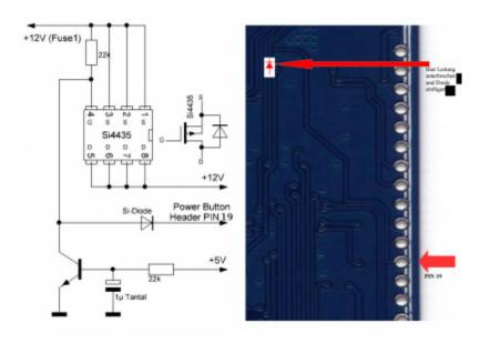
• (RF-04-N-011) The quiescent current through the transmit driver not only flows "also upon receipt" - it flows even when the device is switched off completely (!!!) because the nonsense is, the following changes are made:
