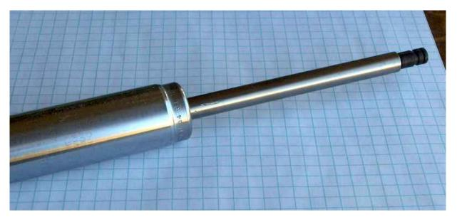
Next, I put couple of washers around the release button at the other end. Normal air springs don't have buttons, so the washers probably aren't needed. I just required a flat surface when the button was depressed, as it doesn't retract completely.
