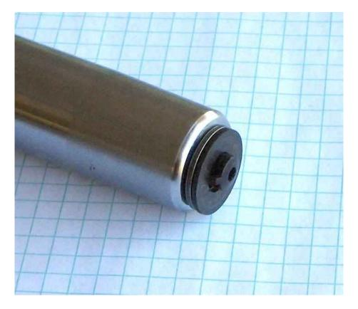
Finally, I put the air spring into a suitable (ie, long enough) gluing clamp. Before tightening the clamp and compressing the air spring, I made sure that the groove was facing down toward the table. I also placed a rag atop the air spring, so that any oil or whatever wouldn't fly around.
