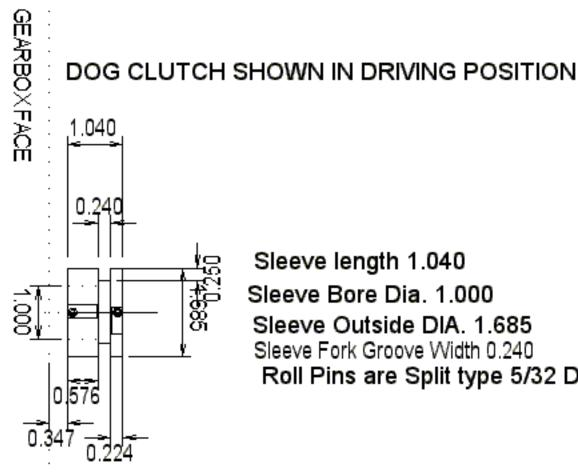
Sleeve length 1.040 Sleeve Bore Dia, 1.000 Sleeve Outside DIA. 1.685 Sleeve Fork Groove Width 0.240 Roll Pins are Split type 5/32 DIA.
