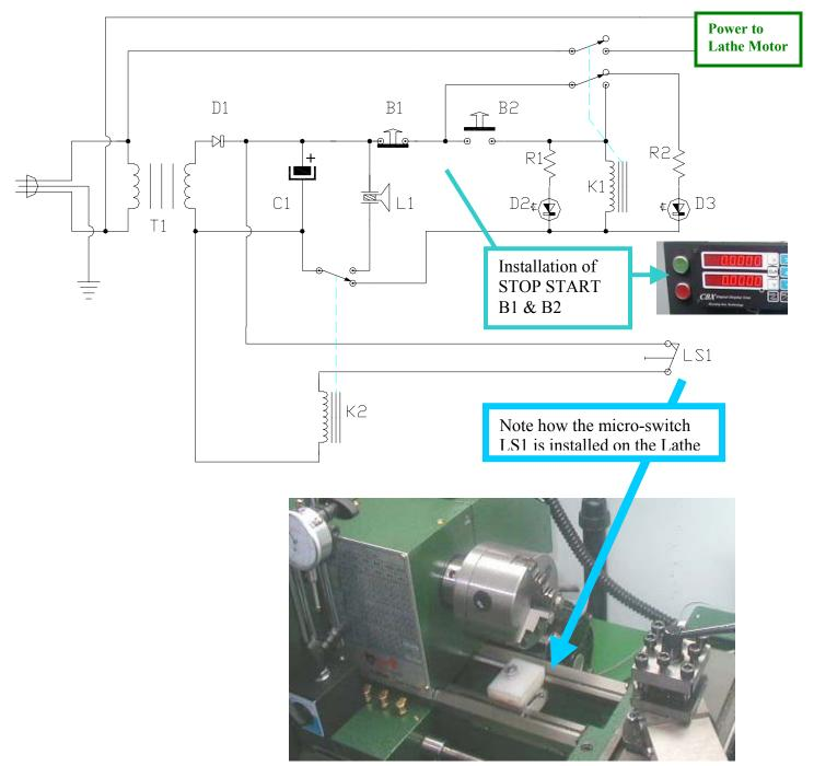
Here is my simple solution to avoid the development of an intimate relationship between a moving tool and a rotating chuck in the 9x20 lathe.
