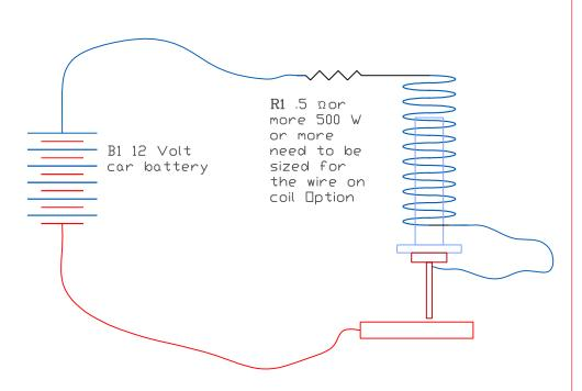
Poor mans EDM using a battery or other power
