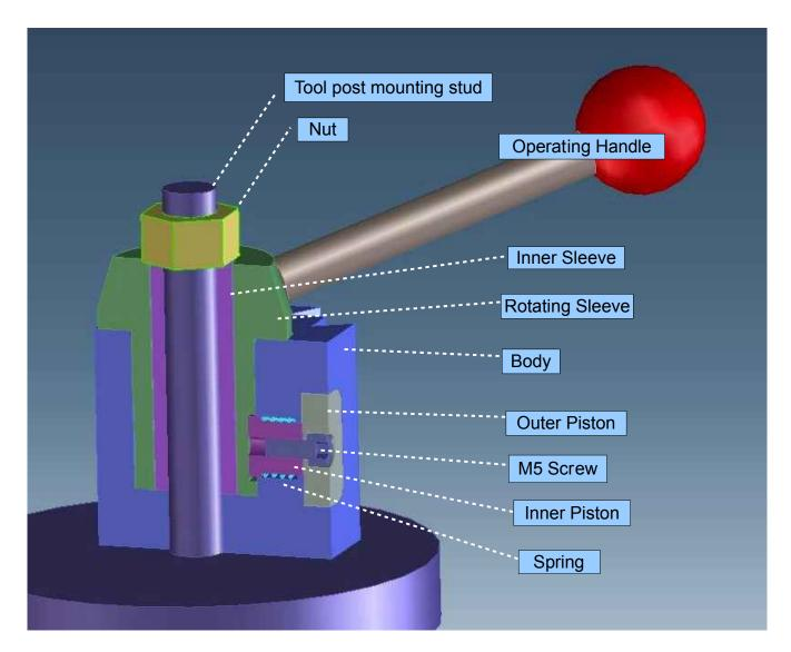
The inner sleeve itself is pretty simple. It just has to be taller than the rotating sleeve, slip over the mounting stud and slip inside the rotating sleeve. If the ID of the inner sleeve is sloppy on the stud and the OD is too close a fit inside the rotating sleeve, it can sometimes jam sideways against the rotating sleeve when the nut is tightened, preventing free rotation. If this is the case, the OD of the sleeve should be reduced slightly.
