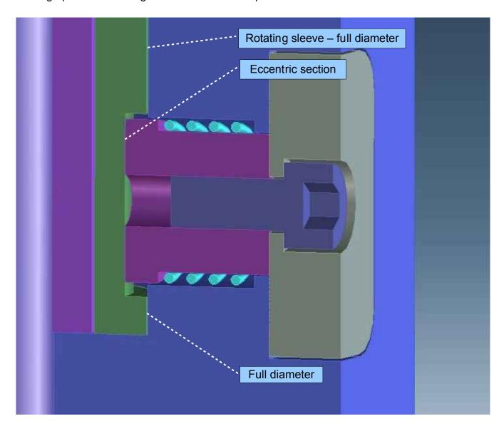
Disassembly of the QCTP (once it's been taken off the lathe) starts with removal of the rotating sleeve. There are two ways to do this:
