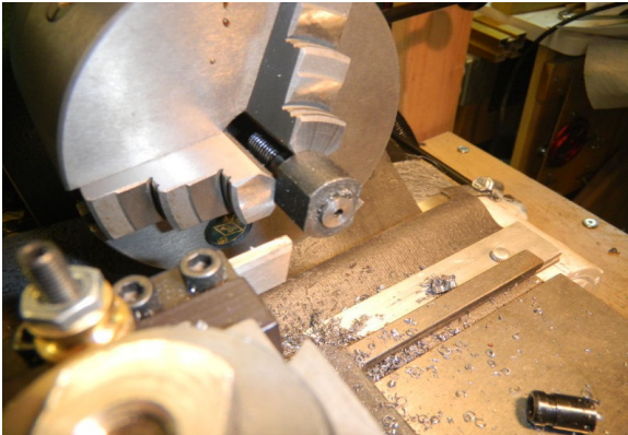
Mount 'a' Gear Shaft on lathe; Part off Shaft
