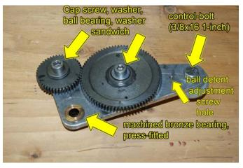
supports, the pivot shaft and the control bolt. I used acetal, an engineering plastic which exhibits very low frictional properties, well suited for my purpose. Please note that I milled away one section of the acetal washer to clear the bracket for my two eccentrics (refer to the photo at the end of this monograph). I didn't want to use a smaller diameter washer as I wanted as much support as I can get to support the control end of the tumbler carrier.
