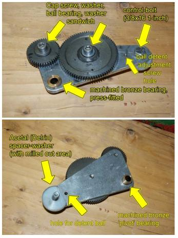
inch bolt and carefully feed the carrier into the lathe so that the pivot shaft can be threaded into the headstock. DO NOT tighten completely, just SHORT of finger tight. The 3/8 inch bolt must exit the arc'ed slot that is cut into the sheetmetal panel.
