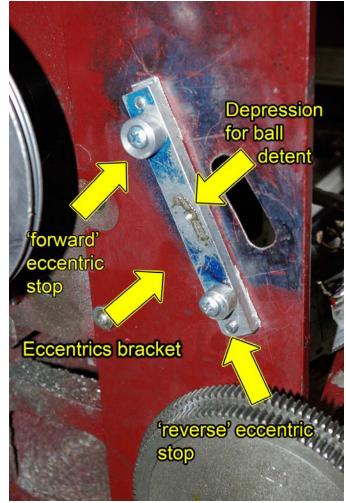
from the lathe, used my center punch and laid out a series of closely spaced marks. Using these marks, I drilled out the arc and finished it off by filing.
