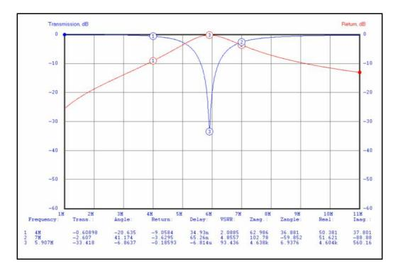
The graph above shows notch depth for the toroid and 890 pF capacitors and was made using an analysis program called Elsie. The notch depth matches closely with measured values.
