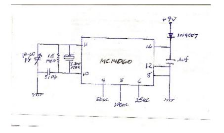
This homebuilt marker was built on a small Radio Shack PCB. The 3.200 Mhz Xtal and MC14060 IC were purchased on ebay for pennies. One hole was bored to mount the PCB in the same position as the original Marker.
