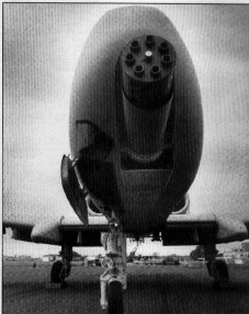
The business end of this A-10 Close Support aircraft with its awesome 30mm GAU-8 Gatling gun, firing depleted-uranium ammunition to kill enemy tanks. Credit: Fairchild Republic Co.
