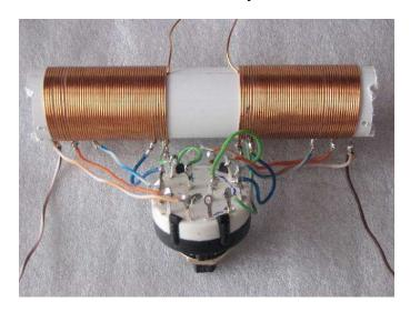
Mount the coil, switch and balun in a suitable box, connecting the ends of the coils to suitable sockets for the dipole legs (I used SO239s, as I drilled the PL239's to take a key ring to accept nylon cord when using it as a "wire dipole") and the inner ends of the coils to the balun.
