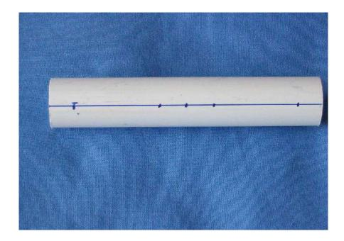
First stage is to cut a 100mm length of 20mm OD conduit, and then mark the centre, and from the centre points 10mm and 42mm out from the centre. Then drill 0.8mm holes through the four outer marks. (ie not the centre mark). Drill right through both sides of the conduit.
