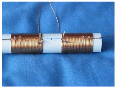
Once you have finished winding the coils, hold them in a vice with something to protect the enamel (I used a piece of bicycle inner tube) and one at a time, open up the taps, clean the enamel off the wire, and re-twist the taps making a neat job of it this time.
