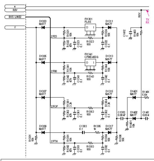
If filter blow-by is a problem when using narrow CW filter option, remove D1309 or D1317. This will remove the "no filter" bypass circuit and eliminate capacitive coupling through the diodes to the rest of the IF chain. These diodes are on bottom of the board near the option filter position. They are MA77 diodes if they are needed later for replacement. de K0ZL
