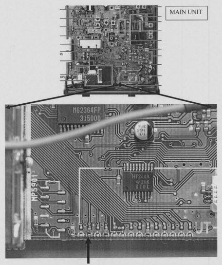
ADD DIODE AT THIS POINT AS SHOWN (cathode to board edge)
