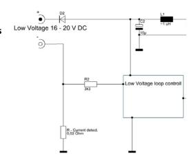
A depleted SLA battery need to be recharged at a slightly greater voltage, around 14,4 V but with some limitation to the current. The theory say that the charging current must not exceed C/10, wehere C is the nominal capacity of the SLA (for a 7 Ah battery, C is 7 A, therefore, the charging current is around 700 mA).
