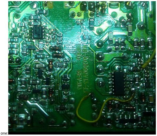
You can notice the separation between the two circuits. (In this picture, the SMPS is not the one I modified because I have the ideea to write this AFTER I pack the SMPS and I glued it! This SMPS has two optocouplers, one for voltage and one for overcurrent protection but the general principle is the same)
