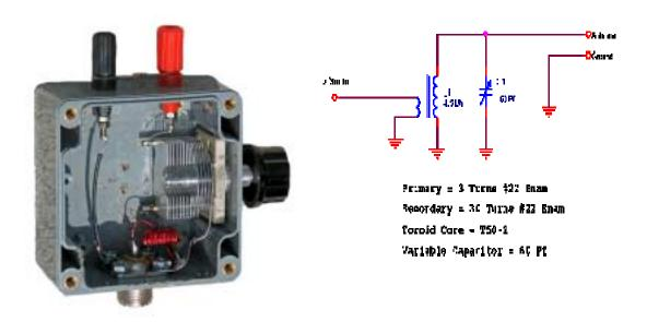
This tuner is about as simple as it gets. It's just a resonant parallel tuned circuit designed to match a High Impedance antenna to a 50 Ohm source impedance at the frequency of interest.. Unlike a Un-Un, Balun or Transformer Matching Device, turns ration is not a factor. The only requirement is to resonant a parallel tuned circuit with a reasonable "Q" so as to be able to tune the circuit while watching a reflectometer for minimum reflected power or VSWR
