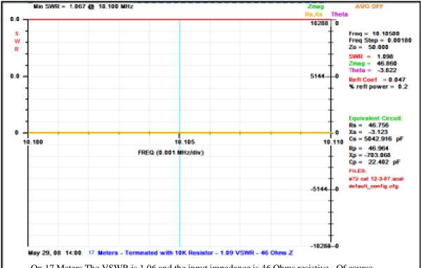
On 17 Meters The VSWR is 1.06 and the input impedance is 46 Ohms resistive. Of course the tuner works across the entire band.
