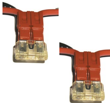
Figure 8 — Anderson Powerpoles rigged as an automotive ATC/ATO fuse holder. See the text for an explanation of how to make this fuse holder.
