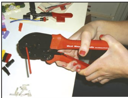
Figure 6 — The author's daughter doing a nice job of crimping Powerpoles using a PWRcrimp tool.
