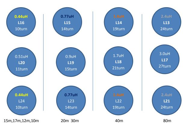
NB Turns may need to be adjusted to reach the exact uH value as listed on the schematic Malcolm G4IHZ
