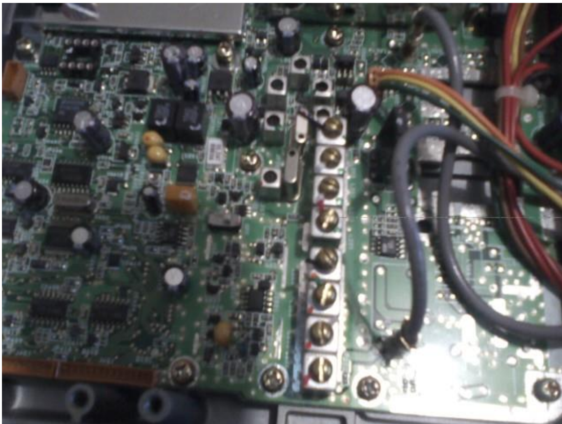
Brass Screws In Coils After Tuning.
