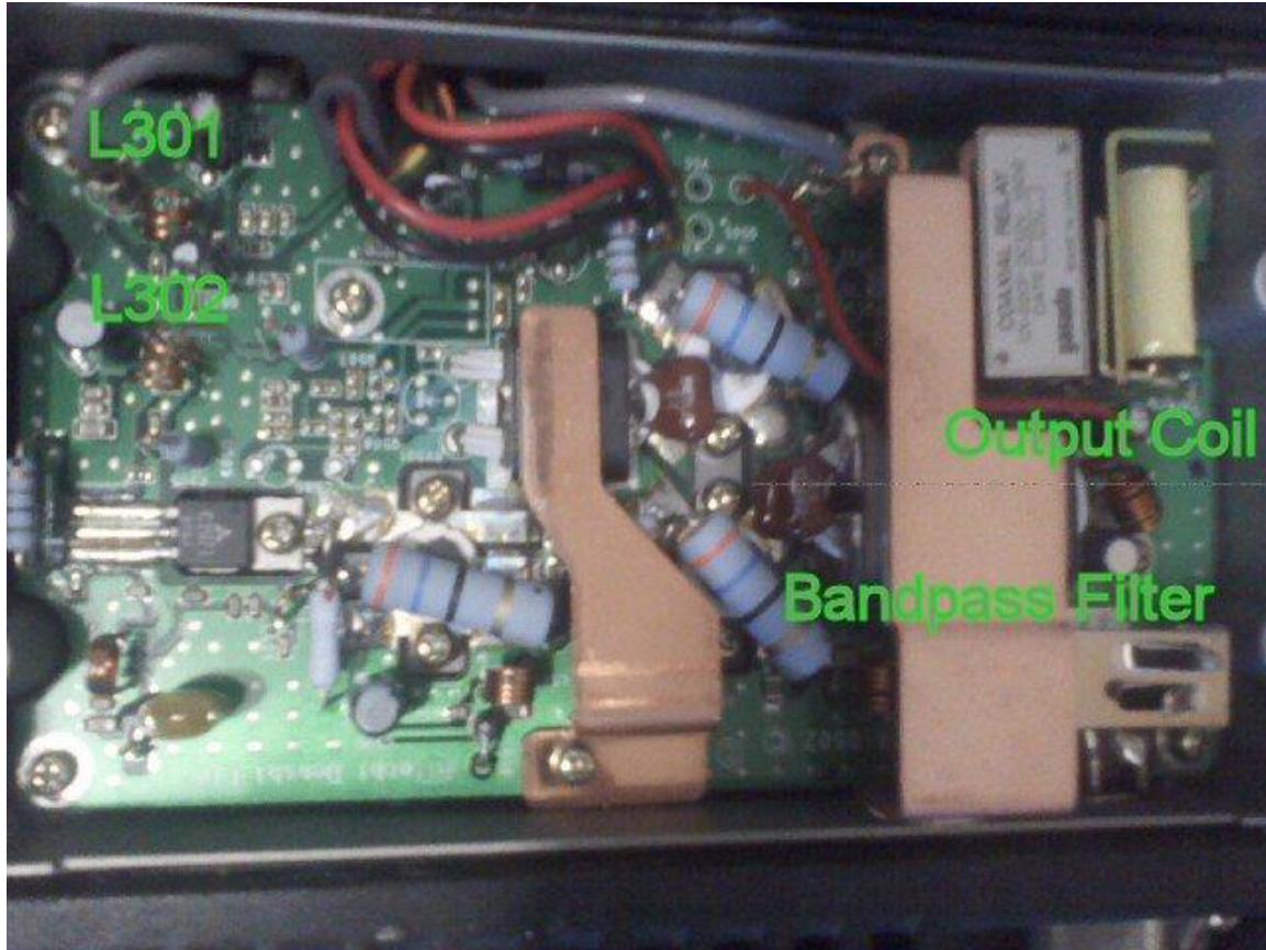
Transmitter Coil Adjustment Locations – Amount of Adjustment Varies Between Radios
