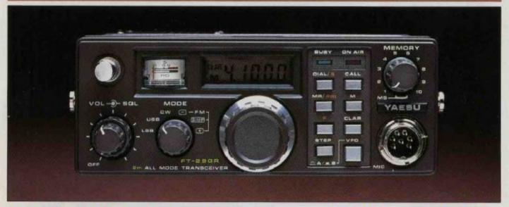
Yaesu is proud to announce a new concept in VHF operating. The FT-290R and FT-690R are fully self-contained portable transceivers, providing multimode performance from a battery-powered package smaller than many FM-only units. Powered by Ni-Cd or alkaline C-cells, these transceivers boast a power output of 2.5 watts minimum, for extended range under field conditions.
