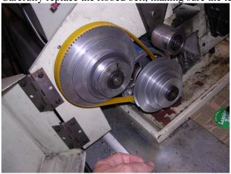
9. Apply a little tension to the belt and tighten the two 17mm lock bolts.
