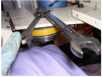
10. Replace V-belt, tighten the 14mm tensioner bolt, replace all covers, etc.
