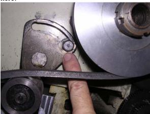
3. Remove V-belt (I rolled mine off while slowly turning the big pulley by hand).
