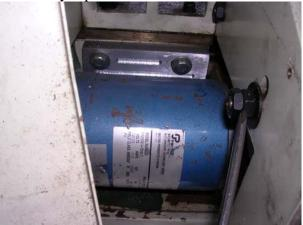
8. Carefully replace the ribbed belt, making sure the teeth seat in the two ribbed pulleys.
