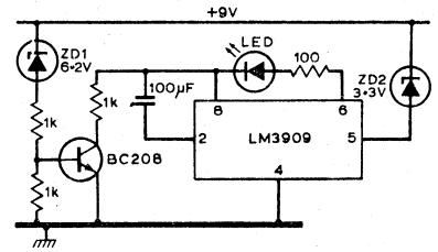
Combined panel light and battery indicator circuit using low duty cycle to reduce battery drain, and with noticeable flashing when voltage drops below a pre-determined Acknowledgements to RADIO COMMUNICATION May 1978.
