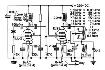
This transmitter is very stable and will deliver up to seven watts of power. Do not be put-off by valves as they are VERY easy to work with and it seems that there are quite a few valves around. Because no-one wants these obsolete things they may be bought for next to nothing at radio rally's. If you are not too particular what type of valve you want then there are lots of valves available.
