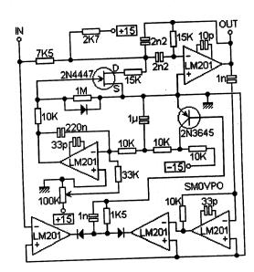
"QRP" receivers and transmitters, for HF CW are often based upon VFO tuning which can be a problem, especially when using the higher frequency bands. I have found that frequency drift is quite annoying at the best of times, but back in 1972 I found this little circuit. It is a narrow band-pass filter, based upon the LM201 OP-Amp. The circuit should work using other OP-Amps, but I have not tested this; I only used the LM201.
