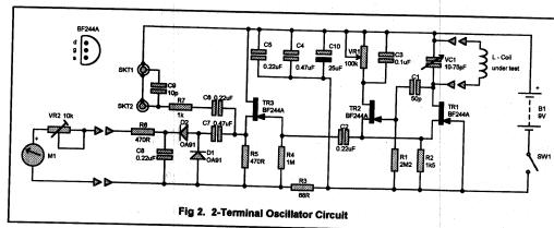
advantages that a) coils can be tested in a practical circuit at the operating frequency and b) measurements are just as easy to make on toroids and sealed coils such as IF transformers as they are on open coils. An additional bonus is that the circuit can be used for a variety of other purposes such as a signal generator, a dip meter or to measure small capacitors.
