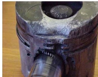
Figure 2: Damage to piston crown.
