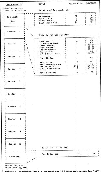
Figure 1. Standard IBM34 Format for 256 byte per sector for 5¼" floppy discs.
