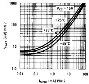
**Discharge Transistor (Pin 7) Voltage vs Sink Current**
