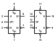
$V_{CC} = Pin 16$ GND = Pin 8
