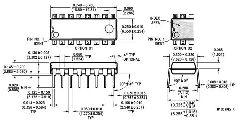
16-Lead Molded Dual-In-Line Package (N) Order Number DM74S109N NS Package Number N16E
