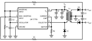
FIGURE 1. RS-232 Power Supply (See Table I, Parts List)
