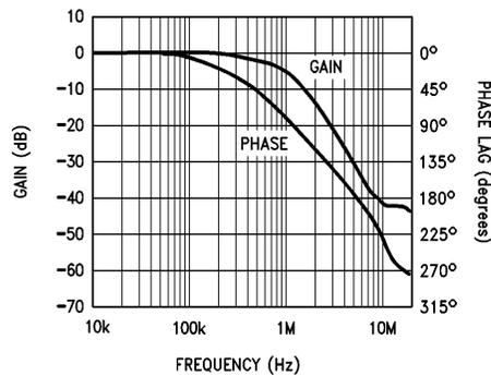
FIGURE 7. Frequency Response of Low-Pass Filter (Reference Figure 6)
