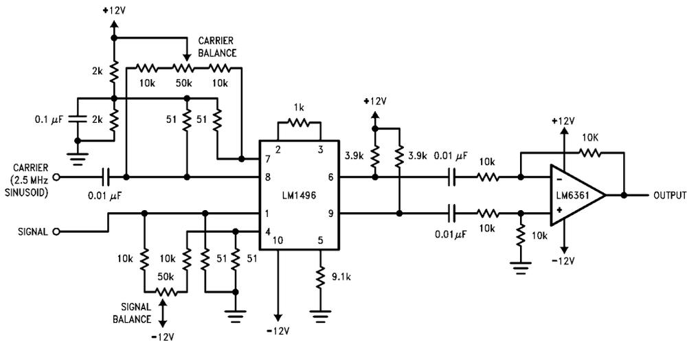
FIGURE 8. Modulator with Single-Ended Output Centered about Ground
