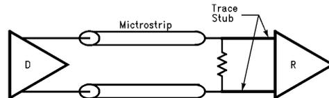
FIGURE 7. A Point-to-Point Configuration Using LVDS
