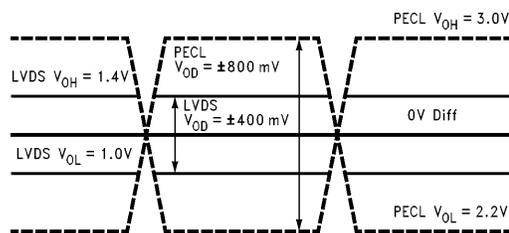
FIGURE 1. PECL vs LVDS Signal Swing
