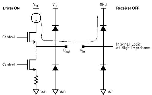
**FIGURE 5. Driver ON and Receiver OFF**
