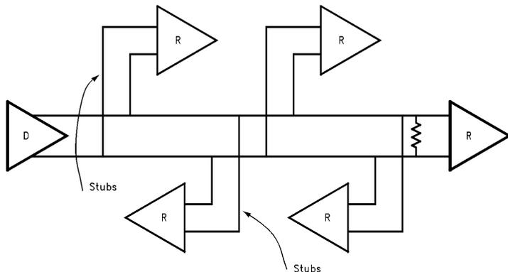
**FIGURE 9. Multi-Drop Configuration for LVDS**
