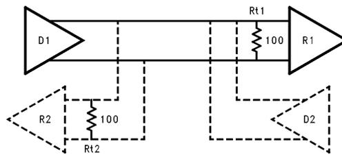
FIGURE 8. Bi-Directional Application over One Pair of Twp
