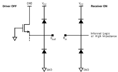
**FIGURE 6. Driver OFF and Receiver ON**
