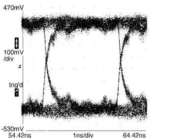
**FIGURE 10a. Eye Pattern at Driver Output**
