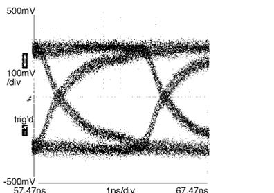
**FIGURE 10b. Eye Pattern at Receiver Inputs with 10m Cable**
