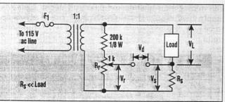
1. THE LOAD'S power factor, which is the cosine of the phase angle between the voltage across the load and the load current, can be calculated simply with this circuit. A 1:1 isolation transformer is used to prevent direct contact with the line.
