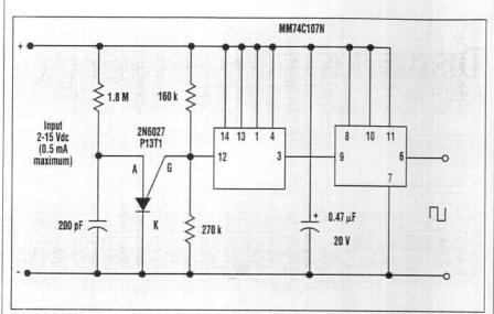
USING THIS CHOPPER CIRCUIT, any dc voltage source in the 2-to-15-V range can be chopped into a unipolar square wave with a peak amplitude that's nearly equal to the dc source voltage, thus creating a known ac voltage.
