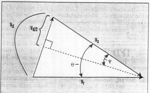
2. BY PROPERLY ADJUSTING  $R_r$ , the vector diagram of voltages  $V_s$ ,  $V_d$ , and  $V_r$  forms an isosceles triangle, which simplifies the power calculation.
