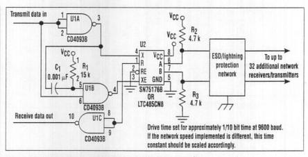
A COLLISION-BASED RS485 NETWORK'S speed can be increased by eight times using this setup. The circuit helps drive the cable to the Mark state by forcing the network driver on for the first 1/10 of a bit time during a Mark. This forces the network back to its resting condition without interfering with collision detection.
