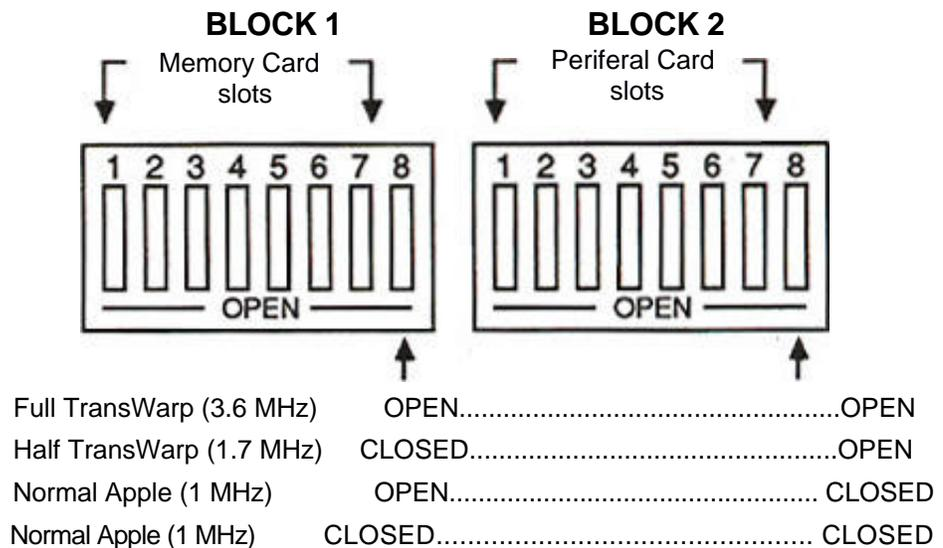
**Figure 2 Sample Switch Configuration for Apple //e System**
