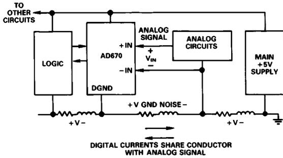
Figure 4b. AD670 Input Rejects Common-Mode Ground Noise
