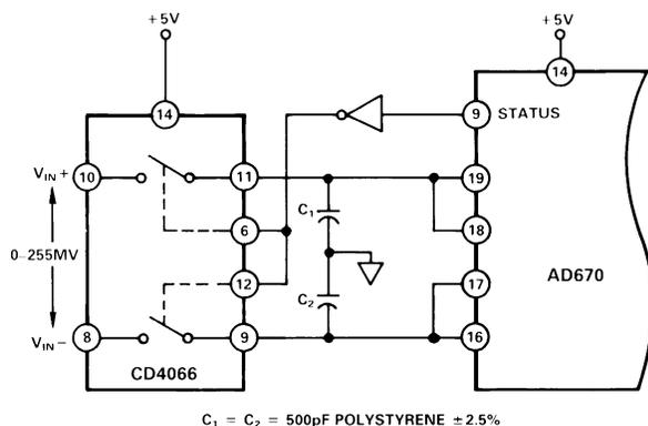
Figure 17. Low Cost Sample-and-Hold Circuit for AD670
