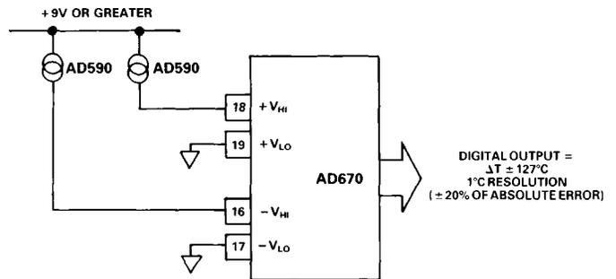
Figure 14. Differential Temperature Measurement Using the AD590
