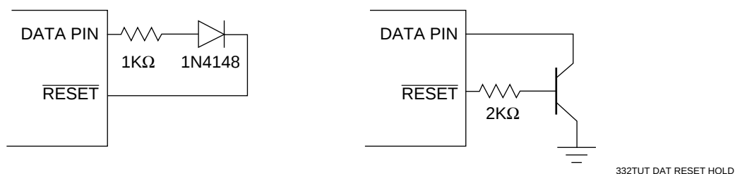
Figure 2 Alternate Methods of Conditioning Data Bus Pins
